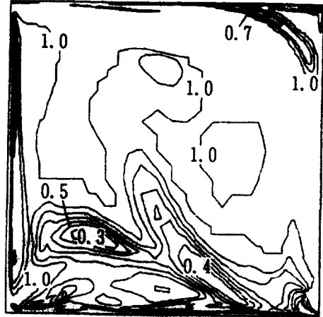
Fig. 15. Distribution of f_{BV} (improved k-\epsilon with f_\mu, f_{BV} and f_{B0} ).
